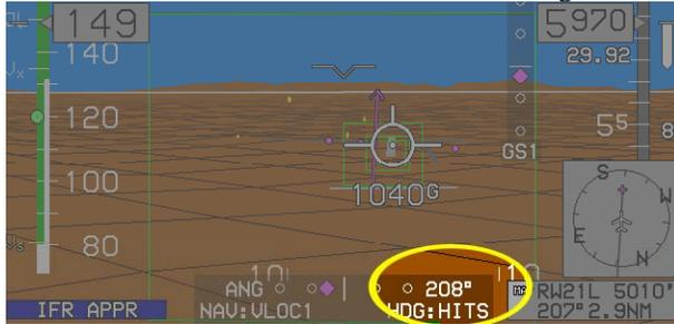
6. Check settings at the bottom of the PFD. In this example:
